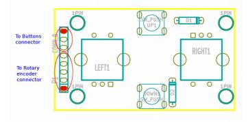
It connects to two connectors on the main board – 'Rotary encoders connector' and 'Buttons connector' (pin 4 of this connector is not used).
