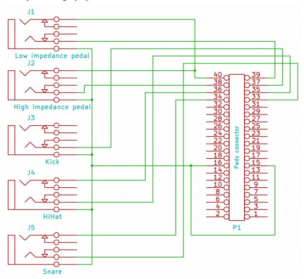
The rest of input jacks are wired to Pads connector 1 and Pads connector 2 as exampled above using Pads connector pinout.
